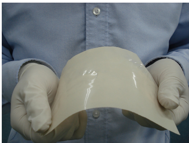
Fig. 2. Optical image of an NPS/SPEEK composite membrane.
